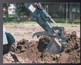
Optional clamp provides added versatility by allowing picking and placement of materials such as logs and rocks.
