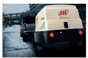
Compact design and smaller footprint make these compressors easier to tow and more maneuverable in tight areas. Aerodynamic design conserves fuel during towing.
