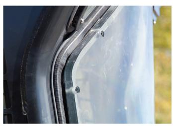
Designed to protect you, and your investment, in the toughest conditions, the forestry applications kit must be installed on the loader in order to operate the forestry cutter attachment. The exclusive forestry door protects you from flying debris and objects. Other benefits include ISO 3449 Level II Falling Object Protective Structure (FOPS) and debris guards for muffler, lights and hydraulic components.
