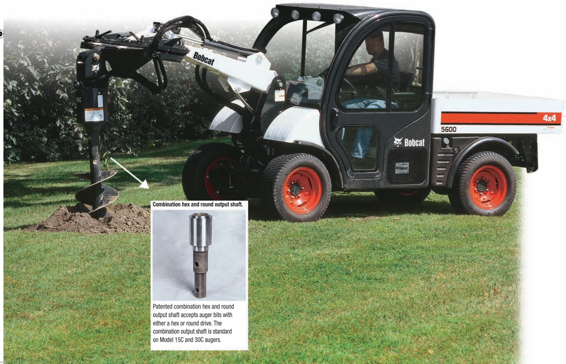
A unique knuckle joint design allows the auger to dig vertical holes even if your Bobcat unit is on uneven terrain.
