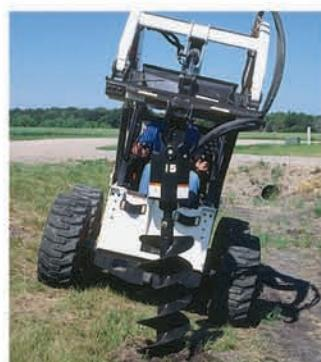
Turn your Bobcat 323, 325, 328, 331, 334, 337, 341, 331E, 430 or 435 compact excavator into an auger machine to drill holes for posts, poles, piers and footings in those hard-to-reach places.
