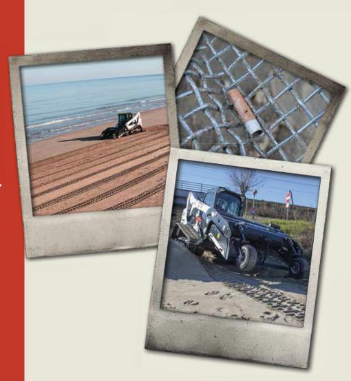
The back blade attached to the back of the machine will insure a nice finish by removing the tracks marks.
